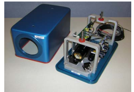
Fig. 3. Laser-based item monitoring system for high-value storage environments.
